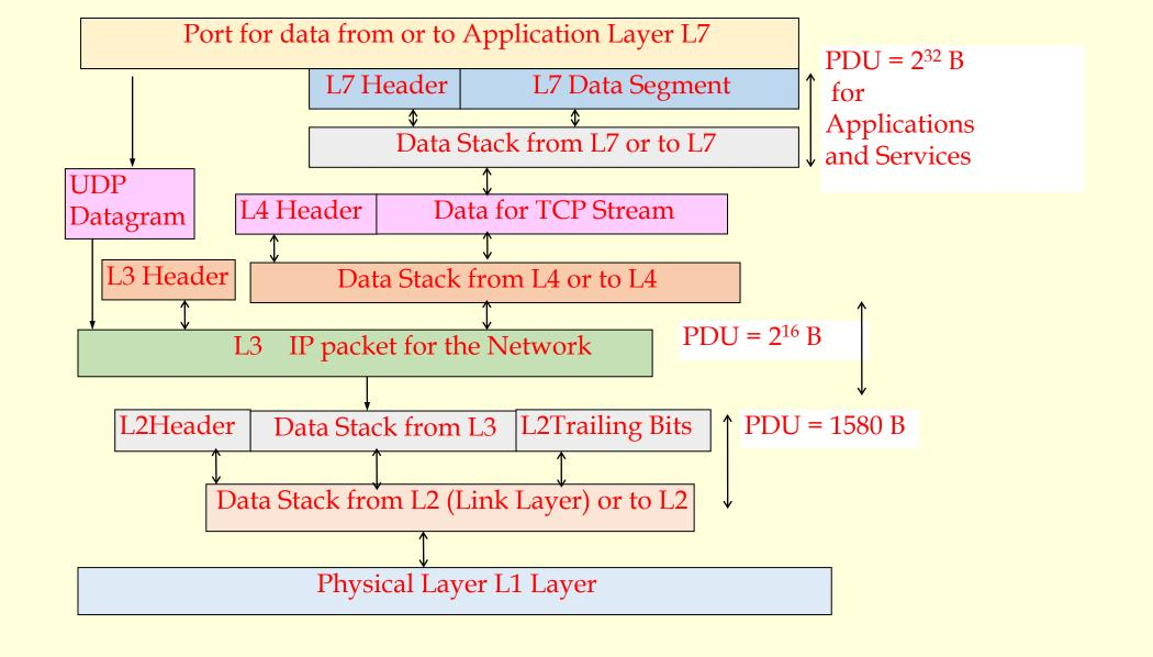
Fig. 4.2 TCI/IP suite four layers model generating data stack for the network, and for physical layer during Internet communication
